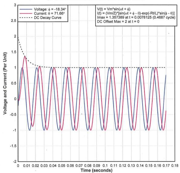
Notes: When  $(\phi - \Theta)$  is 90° and  $\phi$  is not 0°, maximum DC offset of 2.0 pv is produced, but does not result in maximum possible value of current.
