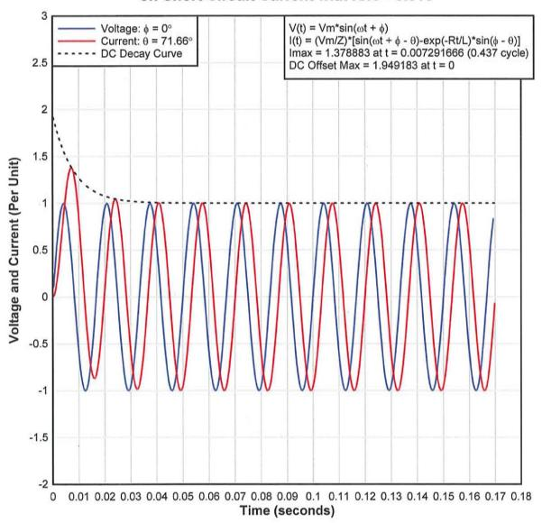
Notes: Maximum value of current is only produced when  $(\phi - \theta)$  is  $\pm 90^{\circ}$  and  $\phi = 0^{\circ}$  or  $\phi = 180^{\circ}$
