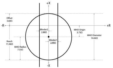
A 78-Element time delay setting will be replaced with functionality that prevents the 78-Element from tripping until the 78-Swing exits the impedance characteristic to minimize the clearing energy that will occur in the generator circuit breaker.
